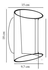
Voltage (V): 220-240 Volt IP degree: IP54 Class (Class 1, Class 2, Class 3): Class 1 (Earth contact) Socket type: LED Module Parallel connection: True
