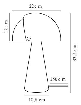
Voltage (V): 230 Volt IP degree: IP20 Maximum bulb wattage (W): 25W Class (Class 1, Class 2, Class 3): Class 2 (Double isolated) Socket type: E27 Switch placement: On the cable
